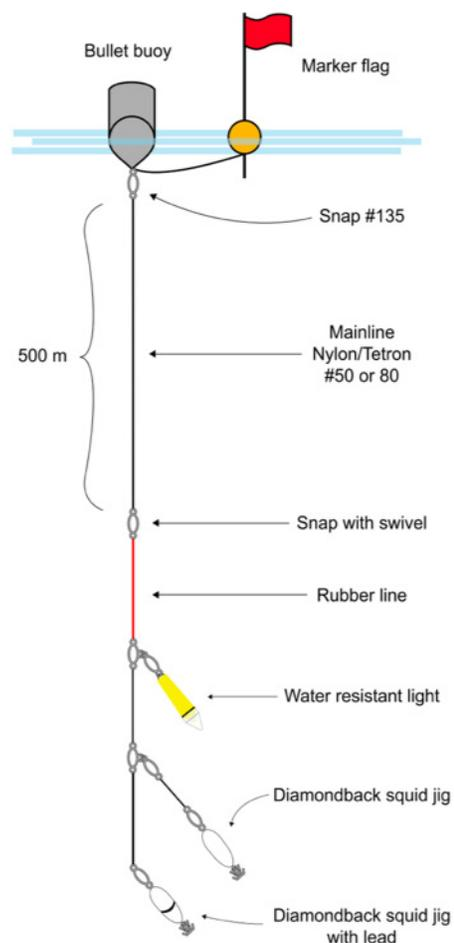
**Figure 6.** A diagram of the dropline gear used in the diamondback squid fishery. Figure from the Ministry of Fisheries, Marine Resources, and Agriculture (2020b).
